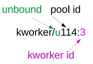
Created: at boot Per-CPU: yes Fixed # pools: yes Fixed workers/pool: no Can migrate: no Persistent, CPU-intensive Created: at boot and dynamic Per-CPU: no Fixed # pools: no Fixed workers/pool: no Can migrate: yes **BUG: workqueue lockup** - pool cpus=1 node=0 flags=0x0 nice=0 stuck for 207s!
