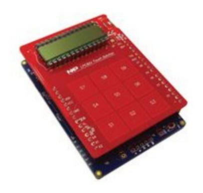
OM13081 - Evaluation Module, Sensing, Touch, Proximity, Capacitive Touch, 8bit Touchpad w / 9 Keys, LCD
