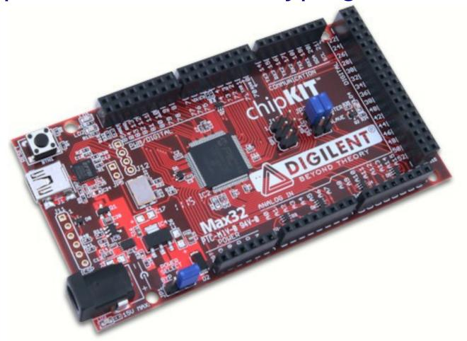
32-bit MIPS processor, Arduino pin-compatible, open toolchain, two CAN controllers, \$50
