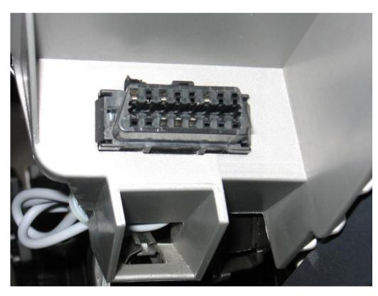
OBD-II connector on left of steering wheel
