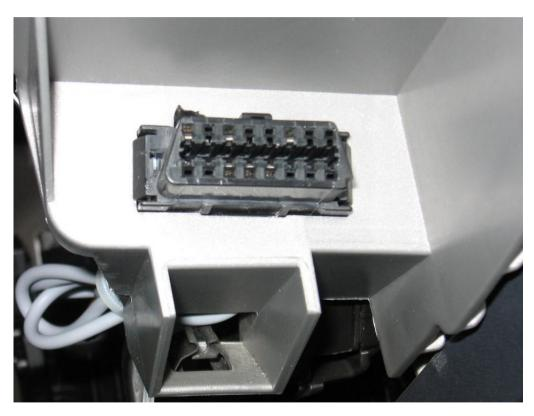
OBD-II connector on left of steering wheel
